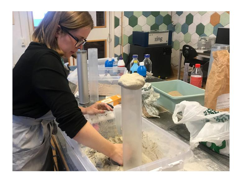
Fill up your tube (clean tube to begin with) by creating fist-size clay balls which you push into the container.
