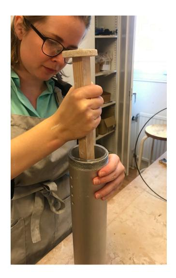
Lower the tube of clay into the container and use a tool to push the clay forwards, into the bottom of the container.
