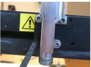
Start by screwing on the connector for the container and the extruder. Use all available 3 screws.
