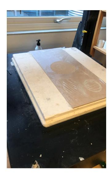
Prepare a print bed. Use an MDF board or such, cloak it with cling film which you attach with tape.
