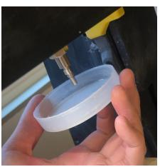
How to use the controller to prime the extruder. Be ready with a container for this step!
