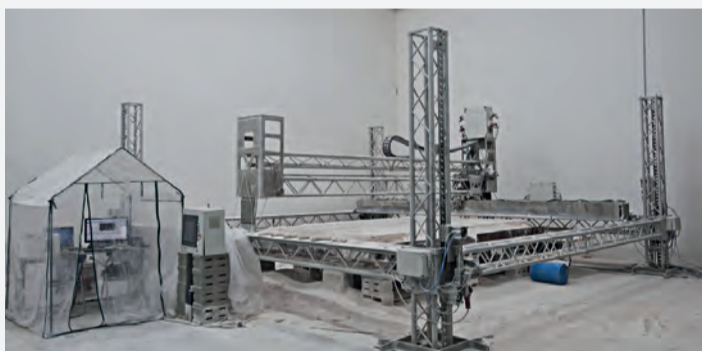
D-Shape printer - one of the first functional construction scale 3D printers created by Enrico Dini.
